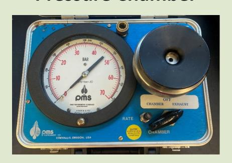
Device to measure water stress of needles by applying a known pressure to the needle
